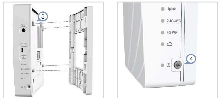
3. With its ports facing down, place the AP over the bracket and then slide it down until it is in its secured position.
